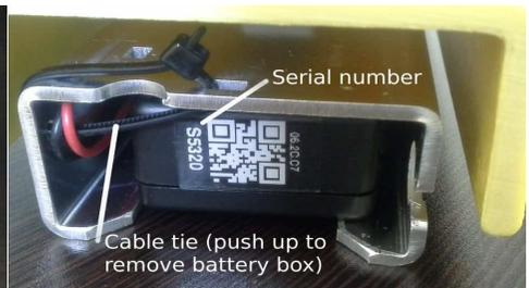
Fig. 4. Close up of battery box
