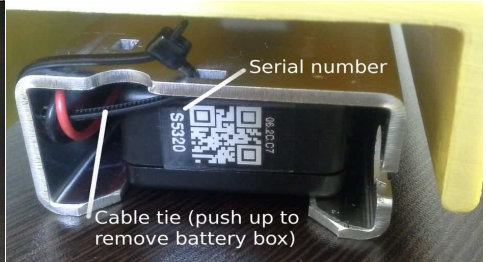
Fig. 4. Close up of battery box
